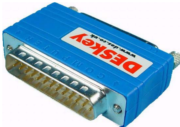
Figure 12: View of SW Security Device
